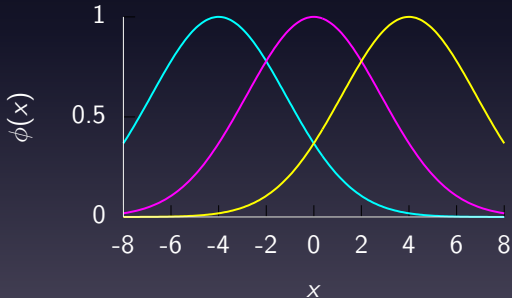
Figure: A set of radial basis functions with width \ell = 2 and location parameters \boldsymbol{\mu} = [-4 \ 0 \ 4]^T .
