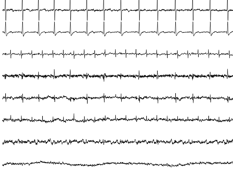
Figure 2: The components uncovered by the GCA algorithm ordered according to the ‘Gaussianity’ of the source. The degrees of freedom parameters were 2.5, 2.5, 2.5, 3.57, 3.79, 6.06, 339 and 832. Components 1, 2, 4 and 5 appear to be associated with the mothers heartbeat, 3 and 6 arise from the fetus. The data appears to only contain six independent components, the other directions being Gaussian.
