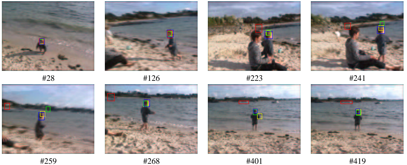
Figure 4: Object tracking results. Tracking the bounding box around the head of the child using the standard particle filter (red), the annealed particle filter (green), and the variational algorithm (yellow). In all cases 100 particles were used. The regions corresponding to the reference bounding box are shown in blue. In the first part of the sequence all three algorithms successfully track the object. In frame 223 the particle filter loses lock due to the colour ambiguity of a nearby region, and never recovers. From time to time the annealed particle filter loses track as well (frames 241 and 259), but is able to recover (frame 268). In contrast the variational algorithm maintains lock throughout, except for a brief period around frame 401 where it moves to the arm of the child.
